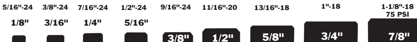
Actual Profile of Compression Threads
