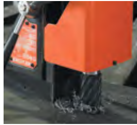
For larger holes, 1/2" and above, use the magnetic base with the standard Weldon shank
