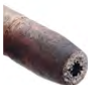
Nozzle fully clogged (not using E-WELD Nozzle)
