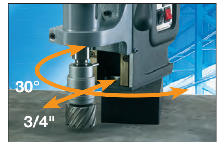
Model MAB 845 features a swivel base providing 30° movement left and right and 3/4" forward and backward.
