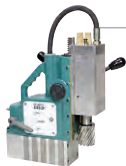
AIRBOR™ AB-4300 p.50 Pneumatic power Capacity: \varnothing 2-1/16" cutter; \varnothing 1/2" twist drill ATEX for hazardous environments
